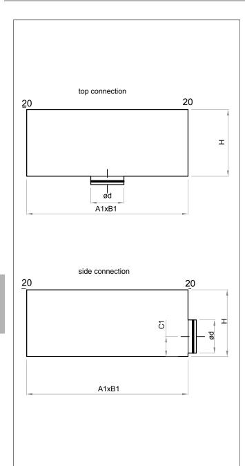
Expansion boxes can be connected to the ventilation installation through the side or top.
